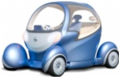
The Pivo 2 has four engines, pivoting wheels, and a rotating cabin so you can face the front while driving in multiple directions. Bumper to bumper "nudge" parking looks like a thing of the past.
